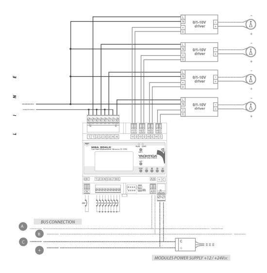
**SCHEME 2: Wiring without relays**
