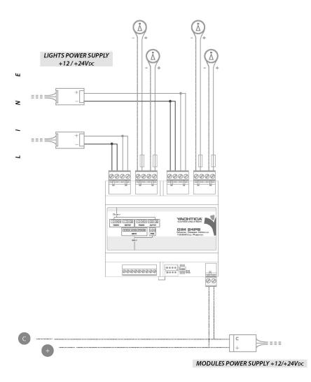
**SCHEME 2: Common negative wiring**
